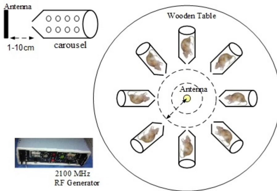
**Figure 1:** Electromagnetic field exposure system (217 Hz pulse modulated-2100 MHz).
